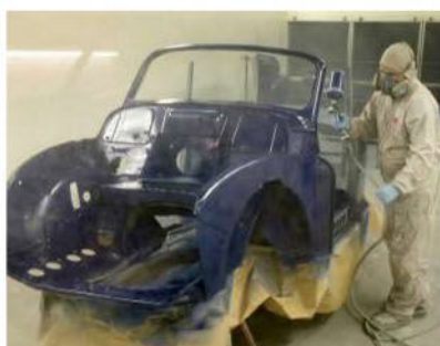
Bodyshell was painted without panels first
