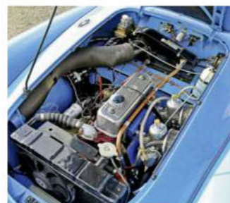
MGB engine boosts performance, electronic ignition and Kenlowe fan boost usability
