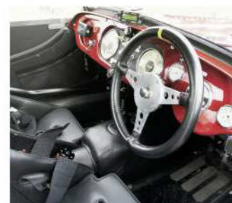
Interior is a tight squeeze; passenger-side harness will need replacing before track time
