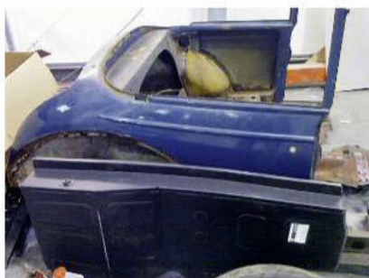
New floorpan ready for fitting – repair patches on the old one were two inches thick in places
