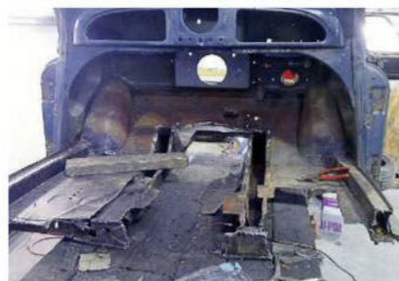
Cutting Minor in half was the easiest way to replace the rotten centre section
