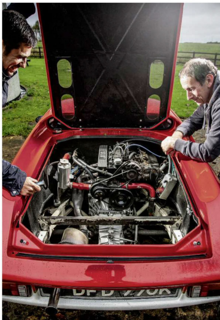
Bored-out cross-flow engine ups power from the original S2's 82bhp to 120bhp
