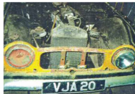
As found in 1990 with missing overdrive, carbs and manifold
