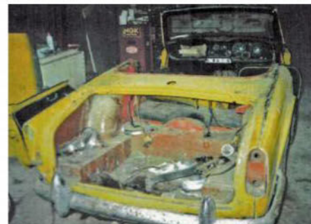
Original red paint still visible on inner wings and boot floor
