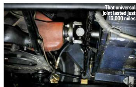
Hatch on the transmission tunnel gives access to the propshaft flange and grease points
