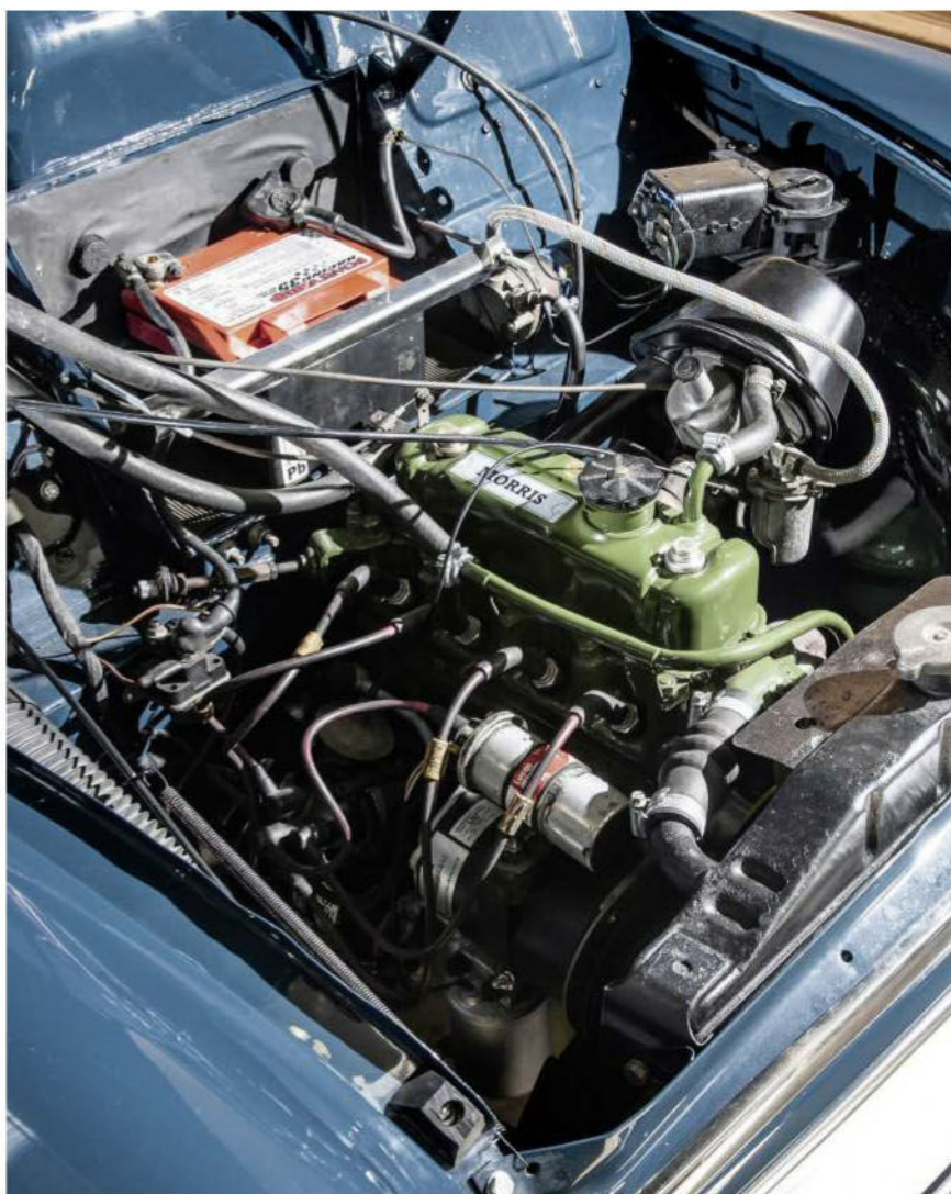
A-series engine looks standard but what looks like a dynamo is actually a Powervamp Powerlite alternator
